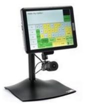
With an Eyegaze system a user can directly select a character by gazing at the letter. Typically used with word prediction.
